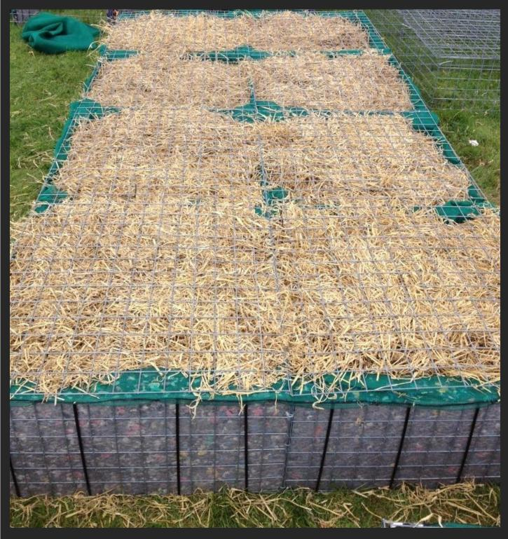
As traditional barley straw applications would seriously disrupt the fishing and sailing due to their footprint, AquaticEngineering proposed using bulk dispensers which would be less disruptive.
